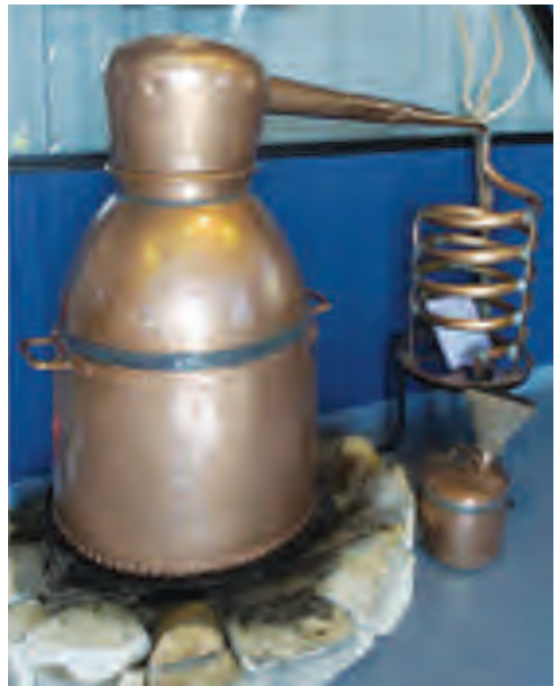
An Alembic : Home distillation unit
