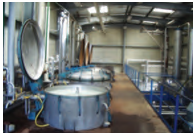
A modern commercial Lavender Distillation Assembly.
