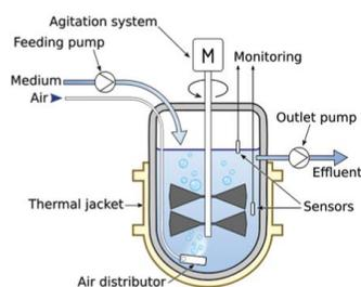
General structure of batch type bioreactor
