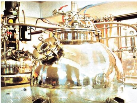
Balloon type bubble bioreactor
