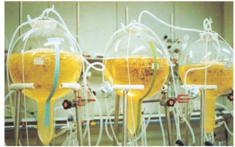
Balloon type air lift bioreactor with root culture
