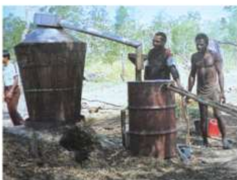
A "Nomadic" type of Field distillation Unit. It is used by Tribes in Irian Jaya for distillation of Eucalyptus Oil.
