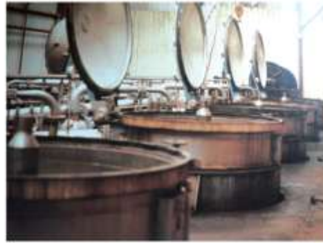
A battery of Stills installed with a multiple condenser system for large-scale distillation (Clove Oil Distillation Factory, Pemba, Tanzania)
