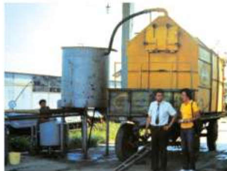
A motorized Still Body that can be transported along the site of cultivation and the harvested material collected en route, and finally brought to a central location for distillation by connecting the flexible steam connection, (Fundulea farm Roumania. At left is Dr. Emil Paun)
