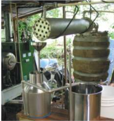
A small-scale modern steam distillation Assembly. In front the Florentine vessels, and on top the Heat Exchanger, open-ended to display the multi-tubes.
