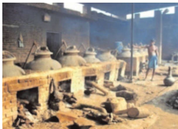
A perfumery in Kannauj showing the Deg-Bhapka technology
